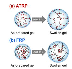
Fig. 2 An illustration of the swelling network structure formed by ATRP (a) and FRP (b)
