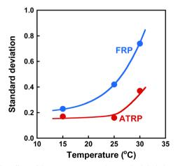
Fig. 8 The effect of the temperature on the standard deviation of  $\langle I \rangle_T$  for the ATRP (red) and FRP (blue) gels. These gels were synthesized with a cross-linker content of 3 mol% at 25 °C.
