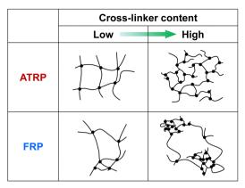
Fig. 6 Tentative illustration for inhomogeneity of ATRP and FRP gels with low and high cross-linker content.
