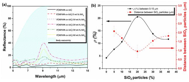
Fig. 1 (a) Evolution of the reflectance in the 5-15 μm range of the PNIPAM-based hydrogel composites as a function of the SiO<sub>2</sub> content, with the human body emissivity at a skin temperature of 34 °C. (b) Percentage of infrared radiation emitted by the human body that is reflected by the PNIPAMbased hydrogel composites (black circles) as well as the distance between the SiO<sub>2</sub> particles (red squares) with respect to the SiO<sub>2</sub> content.
