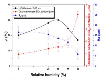
Fig. 3 Relationship between the percentage of infrared radiation emitted by the human body that is reflected by the PNIPAM-based hydrogel composite containing 20 wt% of SiO<sub>2</sub> (black circles), the distance between the  $SiO_2$  particles (red squares) and the surface roughness (blue triangles) with respect to the relative humidity.
