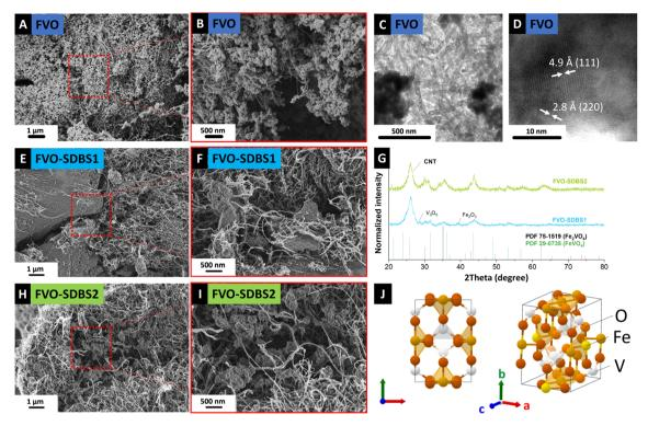
Fig. 3 (A) and (B) Scanning electron micrographs and (C) and (D) transmission electron micrographs of FeV grown in situ on CNT after oxidation, (E) and (F) scanning electron micrographs of FeV with SDBS added to hexacyanoferrate after oxidation, (G) X-ray diffractogram of FVO-SDBS1 and FVO-SDBS-2, (H) and (I) scanning electron micrographs of FeV with SDBS added to vanadyl sulfate after oxidation and (J) crystal structure of FeVO<sub>4</sub>.
