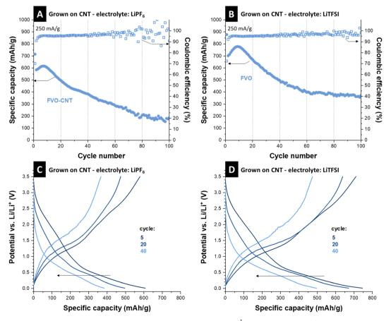
Fig. 4 Stability performances of FVO electrodes at the specific current of 250 mA  $g^{-1}$  in (A) 1 M LiPF<sub>6</sub> in EC/DMC, and (B) 2 M LiTFSI in EC/DMC with their Coulombic efficiencies, and (C) and (D) their respective charge—discharge curves at cycles 5, 20, and 40.
