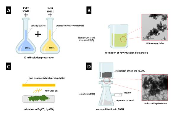
Fig. 1 Schematic representation of (A) and (B) FeV synthesis, (C) heat treatment to FVO, (D) electrode preparation.
