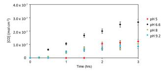
Fig. 5 Evolved CO detected by gas chromatography for PC1|NiO thin films of  $0.79 \text{ cm}^2$  working area with an applied bias of -0.2 V vs. Ag/AgCl under 1 sun AM 1.5, (100 mW cm<sup>-2</sup>) irradiation in various pH buffer solutions as described earlier. Note the pH 6.6 is 50 mM NaHCO<sub>3</sub> solution.
