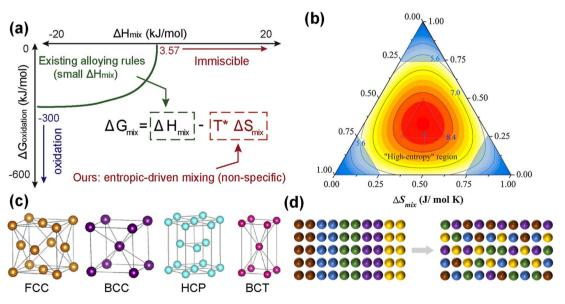
Fig. 1 (a) Enabling more alloy choices based on the entropic contribution ( $-T\Delta S_{mix}$ ). Reproduced with permission.<sup>32</sup> Copyright 2021, Elsevier Ltd. (b) Different spaces of traditional alloy and high entropy alloy. Reproduced with permission.<sup>33</sup> Copyright 2016, Elsevier Ltd. (c) HEAs structure model. Reproduced with permission.<sup>32</sup> Copyright 2021, Elsevier Ltd. (d) High entropy effect.
