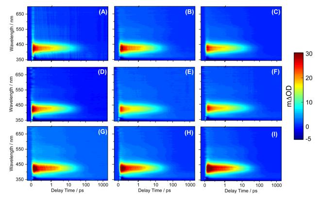
Fig. 4 TEA spectra in caprylic capric triglyceride bulk solution for (A) SM, (B) DESM, (C) DBSM (D) DOSM, (E) DLSM, (F) DCSM, (G) DGSM, (H) DFSM, and (I) DOleySM in the form of a false colour heat map indicating change in optical density (ΔOD). In all cases, the delay time is presented on a linear plot until 1 ps and then as a logarithmic scale between 1 ps and 2 ns.
