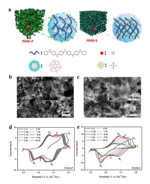
Fig. 1 (a) Microscopic schematic diagram of different PANI doped acids; scanning electron microscopy images of different PANI doped acids: (b) doped phytic acid; (c) doped sulfuric acid; cyclic voltammetry curve (CV curve) sweep rate of 10 mV s<sup>-1</sup> for different PANI doped acids: (d) PANI doped phytic acid electrode in 1 M zinc sulfate electrolyte with addition of zinc phytate (1%); (e) PANI doped sulfate electrode in 1 M zinc sulfate electrode in 1 M zinc sulfate electrolyte.
