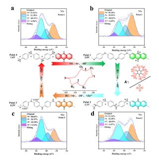
Fig. 3 In situ XPS analysis of N 1s in Zn//PANI cells at different voltages during the second cycle and the electron gain/loss process: (a) point 4; (b) point 1; (c) point 2; (d) point 3.
