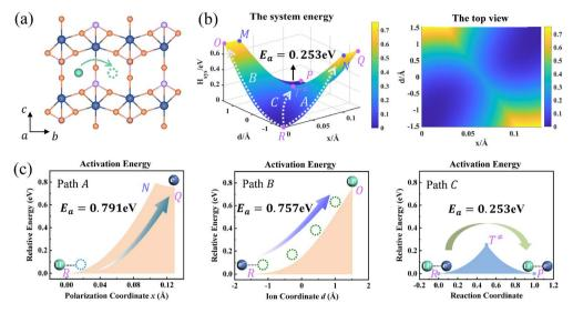
Fig. 4 (a) Structure diagram of  $\text{Li}^+$  hopping along the b-axis in FePO<sub>4</sub>. (b) Potential energy surface based on the Hamiltonian model (left) and its top view (right) for ion hopping and electron transfer. (c) Potential energy curves of paths A, B, and C.
