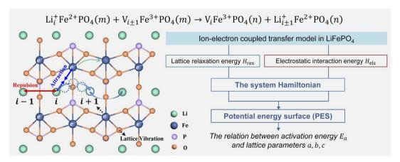
Fig. 1 Schematic illustration of ion hopping and electron transfer in LiFePO<sub>4</sub> and the model framework.
