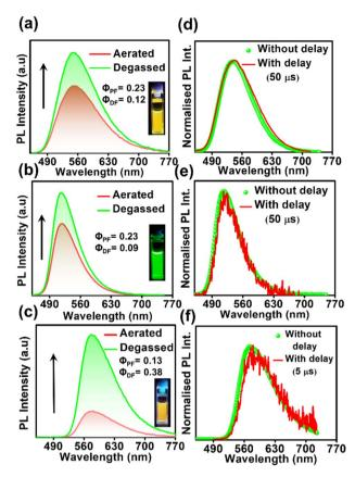
Fig. 2 Emission spectra in aerated and degassed toluene of (a) DPAOCN, (b) DPAMCN, and (c) DPAPCN (for 30  $\mu m$  of luminogen concentration). Steady-state and time-gated emission spectra in degassed toluene of (d) DPAOCN, (e) DPAMCN, and (f) DPAPCN. 2 ms sample windows were used for DPAOCN and DPAMCN, whereas for DPAPCN, a 1 ms sample window was used for gated spectra measurement.
