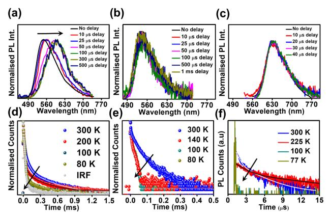
Fig. 5 (a) & (d) Time-gated emission spectra (with varying time delay) and temperature-dependent emission of DPAOCN powder (collected at 550 nm). (b) & (e) Time-gated emission spectra (with varying time delay) and temperature-dependent emission of DPAMCN powder. (c) & (f) Time-gated emission spectra (with varying time delay) and temperature-dependent emission of DPAPCN powder. Sample windows in all cases are kept at 2 ms.
