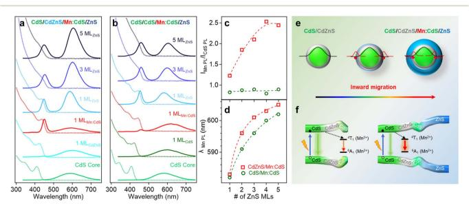
Fig. 5 (a and b) Normalized absorption and PL spectra of (a) CdS/CdZnS/Mn:CdS/ZnS $_{(1-5 \text{ MLs})}$  and (b) CdS/CdS/Mn:CdS/ZnS $_{(1-5 \text{ MLs})}$  core/multishell QDs. (c) The PL Intensity ratio of Mn(II) and CdS host lattice and (d) the changes of Mn(II) PL peak position as a function of ZnS shell thickness. (e) Schematic of the dopant inward migration by inserted CdZnS alloyed trap layer and (f) the band alignment of the CdS/CdZnS/Mn:CdS/ZnS core/multi-shell QDs.
