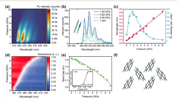
Fig. 1 (a) 2D colormap of pressure-dependent PL intensity and wavelength of the phenanthrene crystal. (b) *In situ* PL spectra of the phenanthrene crystal below 1.65 GPa. (c) Pressure-dependent PL wavelength and intensities. (d) 2D colormap of high-pressure UV-vis absorption spectra of the phenanthrene crystal. (e) Schematic illustrations of the band gap changes. (f) The sketch map for molecular packing of the phenanthrene crystal.
