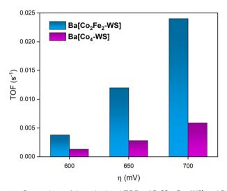
Fig. 9 Comparison of the calculated TOFs of Ba[Co<sub>2</sub>Fe<sub>2</sub>-WS] and Ba [Co<sub>4</sub>-WS] at different overpotentials during RDE-LSV measurements. The experiments were conducted using 30 wt% Ba[POM]/CP electrodes at pH = 7.2 using 50 mM KP<sub>i</sub> buffer and KNO<sub>3</sub> (1 M) as aqueous electrolyte. The scan rate was  $1 \text{ mV s}^{-1}$  and the rotational speed was 1600 rpm.
