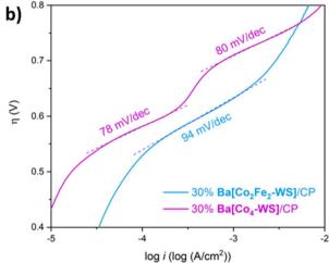
Fig. 8 Comparative OER electrocatalytic activity of 30 wt% POM/CP electrodes.  $Ba[Co_2Fe_2-WS]$  (blue),  $Ba[Co_3W-WS]$  (green),  $Ba[Co_4-WS]$  (purple). (a) Rotating disk electrode linear sweep voltammetry (RDE-LSV). (b) Tafel plots, as derived from the RDE-LSV data. The experiments were conducted in a single-cell using a pH = 7.2, 50 mM KP<sub>i</sub> buffer and KNO<sub>3</sub> (1 M) as aqueous electrolyte. The scan rate was 1 mV s<sup>-1</sup> at a rotation speed of 1600 rpm.
