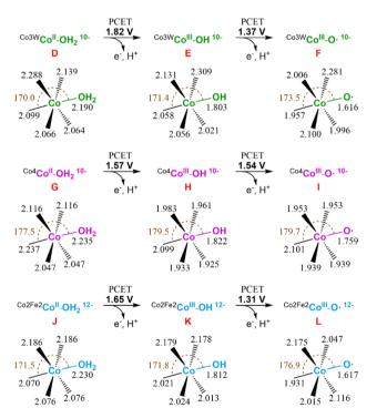
Fig. 11 Schematic representation of the first two PCET events of the water oxidation reaction for the  $Co_3W$ -WS (top),  $Co_4$ -WS (middle), and  $Co_2Fe_2$ -WS (bottom) systems. Potential energies are given in V vs. NHE at pH = 7. Values for the  $Co_4$ -WS system are extracted from ref. 44.
