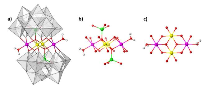
Fig. 1 (a) Polyhedral representation of the structure of  $[Co_2Fe_2-WS]$ . (b) Connectivity within the rhombic cobalt–iron-oxo belt and cobalt heteroatoms. (c) Top view of the cobalt–iron-oxo core structure. Colour code: pink: Co<sup>II</sup> in octahedral geometry; green: Co<sup>II</sup> in tetrahedral geometry; yellow: Fe<sup>III</sup>; red: O; white: H; grey polyhedra:  $\{WO_6\}$  units.
