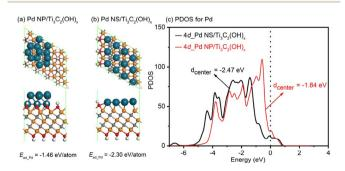
Fig. 6 The relaxed atomic structures of the (a) Pd NP/ $Ti_3C_2(OH)_x$  and (b) Pd NS/ $Ti_3C_2(OH)_x$  models, where the gray, red, white, orange, and blue balls represent C, O, H, Ti, and Pd atoms, respectively. (c) The d-PDOS plots of the different Pd nanostructures in the Pd NP/ $Ti_3C_2(OH)_x$  and Pd NS/ $Ti_3C_2(OH)_x$  models.
