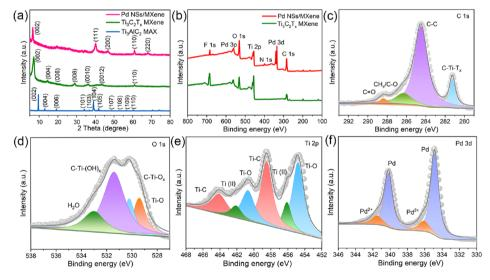
Fig. 3 Structural characterization of the Pd NSs/MXene heterojunction. (a) XRD patterns of the Pd NSs/MXene,  $Ti_3C_2T_x$  MXene, and  $Ti_3AlC_2$  samples. (b) XPS survey spectra of Pd NSs/MXene and  $Ti_3C_2T_x$  MXene. The typical (c) C 1s, (d) O 1s, (e) Ti 2p, and (f) Pd 3d core-level XPS spectra of Pd NSs/MXene.
