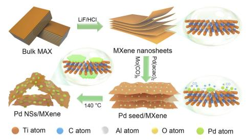
Fig. 1 The synthesis process of the 2D/2D Pd NSs/MXene heterojunction: (1) synthesis of 2D MXene nanolayers by a LiF and HCl etching route; (2) growth of Pd seeds on the surface of MXene as well as the generation of CO molecules by the decomposition of Mo(CO)<sub>6</sub>; (3) gradual formation of 2D Pd nanosheets on the MXene nanosheets.
