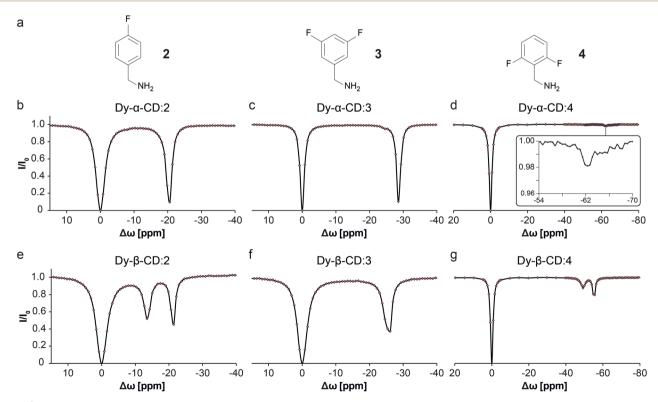
Fig. 4  $^{19}$ F-paraGEST z-spectra for solutions of Dy-α-CD or Dy-β-CD with different guest molecules. (a) The molecular structures of guests 2, 3, and 4. (b-g) Z-spectra of the indicated host (as noted in each panel) and the corresponding guest. The data in panels b-d was adapted from ref. 30.
