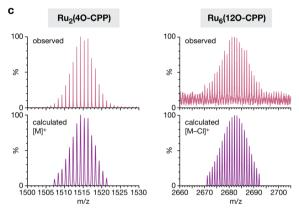
Fig. 4 (a) Synthesis of the diruthenium complex  $Ru_2(Ph_2dhbq)$  from the reduced form of the model ligand,  $H_4Ph_2dhbq$ . (b) Synthesis of the diruthenium complex  $Ru_2(4O\text{-}CPP)$  from the ligand 4HO-CPP. (c) Observed (top, pink) versus simulated (bottom, purple) high-resolution MALDI-TOF spectra of the polyruthenium complexes  $Ru_2(4O\text{-}CPP)$  and  $Ru_6(12O\text{-}CPP)$ .
