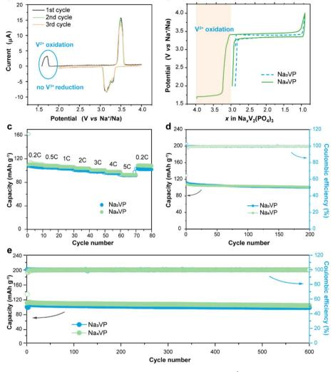
Fig. 5 (a) Cyclic voltammogram profiles of the Na<sub>4</sub>VP cathode at a scan rate of 0.1 mV s<sup>-1</sup>. (b) Initial charge–discharge curves of Na<sub>5</sub>VP and Na<sub>4</sub>VP electrodes between 2.0 and 4.0 V at 0.2C. (c) Rate performance, (d) cycling stability at 0.5C, and (e) long-term cycling stability at 1C of Na<sub>3</sub>VP and Na<sub>4</sub>VP electrodes
