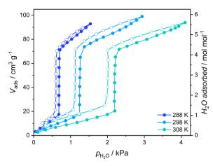
Fig. 3 Vapor adsorption isotherms of water recorded for 1 ( $1.4H_2O$  activated in a vacuum at 323 K). Full circles – adsorption, open circles – desorption.
