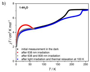
Fig. 7  $\chi T(T)$  variation recorded after 638 and 808 nm light irradiation for 1 (a) and  $1\cdot 4H_2O$  (b). Initial measurements and measurement after thermal relaxation were performed at 2 K min<sup>-1</sup> sweep rate, while measurements after light irradiation were performed at 0.3 K min<sup>-1</sup>.
