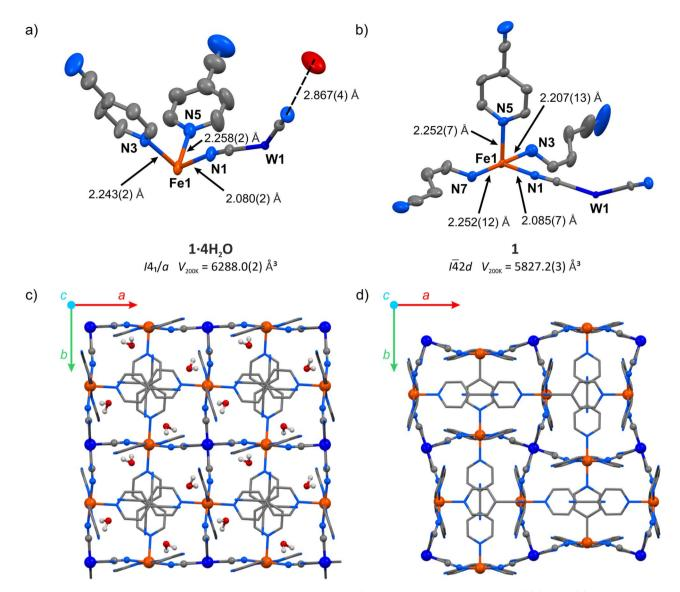
Fig. 2 Structural transformation accompanying the transition from 1·4H<sub>2</sub>O to 1: asymmetric unit of 1·4H<sub>2</sub>O (a) and 1 (b) with selected bond distances (hydrogen atoms were omitted for clarity), as well as coordination frameworks of 1·4H<sub>2</sub>O (c) and 1 (d) as seen along the crystallographic c-axis (hydrogen atoms of 4-cyanopyridine molecules were omitted for clarity). W - dark blue, Fe - orange, O - red, N - blue, C - grey.
