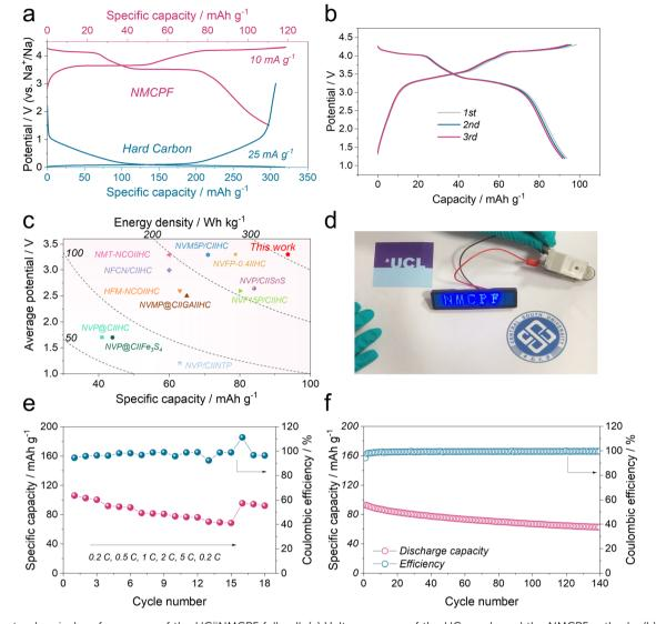
Fig. 5 Electrochemical performances of the HC $\parallel$ NMCPF full cell. (a) Voltage curves of the HC anode and the NMCPF cathode. (b) Charge–discharge profiles of the HC $\parallel$ NMCPF full cell for the initial three cycles at 0.5C (1C = 110 mA g $^{-1}$ ). (c) Comparison of our work with previous reported works. (d) Picture of a LED badge powered by the HC $\parallel$ NMCPF full cell. (e) Rate capability of the full cell. (f) Cycling stability of the full cell at 0.5C.
