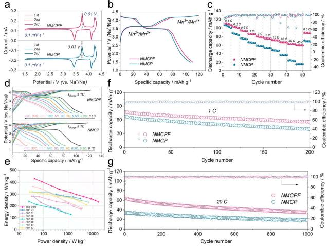
Fig. 4 Electrochemical capabilities within 1.5–4.3 V. (a) CV curves at  $0.1 \,\mathrm{mV}\,\mathrm{s}^{-1}$ . (b) Initial charge/discharge curves at  $0.1 \,\mathrm{C}\,\mathrm{IC} = 110 \,\mathrm{mA}\,\mathrm{h}\,\mathrm{g}^{-1}$ ). (c) Rate properties. (d) Charge/discharge profiles at various rates. (e) Ragone plot. Cycling capabilities at (f) 1C and (g) 20C.
