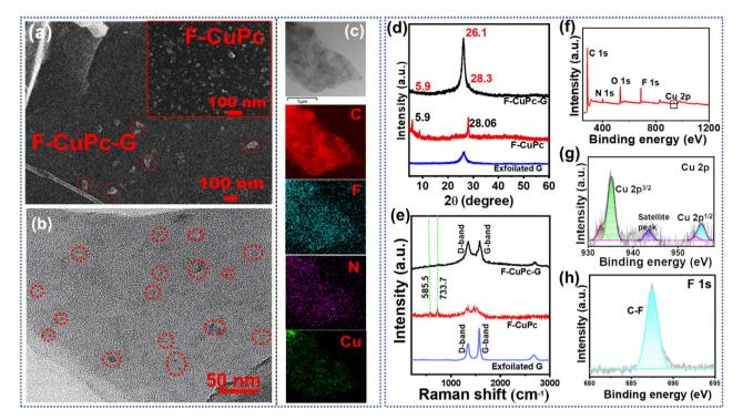
Fig. 4 (a) FE-SEM image of F-CuPc-G; inset: F-CuPc, (b) TEM image of F-CuPc-G; (c) TEM elemental mapping of F-CuPc-G, shows the distribution of C, F, N and Cu; (d) XRD pattern and (e) Raman spectra of F-CuPc-G, F-CuPc and exfoliated graphene. (f) The full survey XPS spectra of F-CuPc-G; high resolution XPS spectra of (g) Cu 2p, and (h) F 1s in F-CuPc-G.
