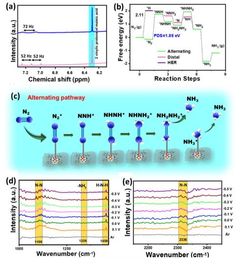
Fig. 6 (a) Isotope labelling experiment displaying  $^{1}H$  NMR spectra obtained after the NRR in 1 M Na<sub>2</sub>SO<sub>4</sub> with  $^{14}N_2$  (pink) and  $^{15}N_2$  (blue) as feed gases, (b) Free energy profile of the NRR for F-CuPc-G, (c) scheme showing the reaction mechanism of F-CuPc-G during NRR follows alternating pathway. (d and e) *In situ* ATR-FTIR spectra obtained for F-CuPc-G.
