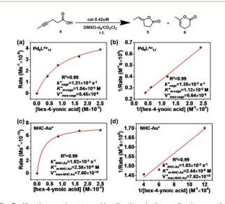
Fig. 7 Kinetic experiments and implications in the cyclization reaction of hex-4-ynoic acid. (a) Kinetic analyses and (b) Lineweaver–Burk plot for the  $\mathrm{Pd_6L^{Au}}_{12}$  cage. (c) Kinetic analyses and (d) Lineweaver–Burk plot for NHC–Au $^+$ .
