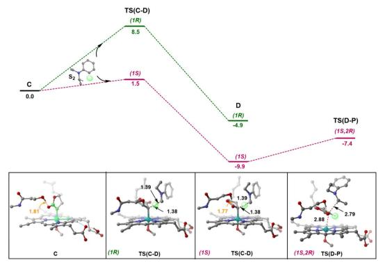
Fig. 6 Total electronic energy profile of L9 (kcal  $mol^{-1}$ ) for HAT and the lowest-energy radical rebound TSs with  $S_2$  approaching from face A are shown. The H atoms (except the ones taking part in H-bonding) are omitted for clarity.
