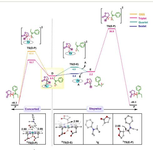
Fig. 2 Gibbs free energy profile (kcal mol<sup>-1</sup>) for comparison of concerted and stepwise pathways for C-H insertion at different spin states of Fe. Distances are in A. The H atoms are omitted for clarity.
