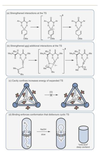
Fig. 6 Catalytic activity due to enhanced TS binding can arise from (a) the strengthened interactions between the catalyst and TS;<sup>118</sup> (b) additional interactions that are specific to the TS;<sup>119</sup> (c and d) conversely, confinement effects can also lead to a higher TS energy, allowing the protection of reactive species.<sup>58,120</sup>
