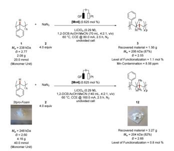
Fig. 4 Scale-up of the C-H azidation on polystyrene. See ESI† for details.
