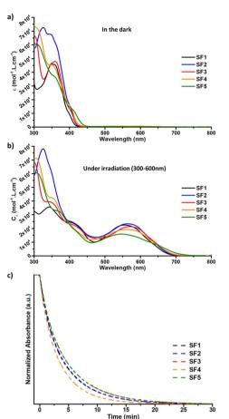
Fig. 2 UV-visible absorption spectrum for SF1, SF2, SF3, SF4 and SF5 without (a) and with (b) under continuous irradiation (Xenon lamp, 200 W, 300–600 nm, orthogonal with respect to the measuring beam). Concentration:  $2\times10^{-5}$  mol L<sup>-1</sup> in toluene at 25 °C. (c) Comparison of normalized discoloration curves of SF1-5 in solution after reaching PSS. Concentration:  $2\times10^{-5}$  mol L<sup>-1</sup> in toluene at 25 °C.
