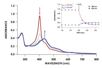
Fig. 4 Reaction of 10  $\mu$ M as-isolated Phe41Ala cyt P460 (red) with 30  $\mu$ M Li<sub>2</sub>O<sub>2</sub> in 20 mM Tris/200 mM NaCl buffer at pH 8.0 and 25 °C. The blue trace represents the final scan and grey traces were recorded every 0.2 minutes. Time courses of the absorbances corresponding to the proenzyme (403 nm) and product (436 nm) are shown in the inset.
