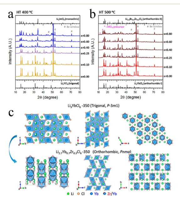
Fig. 8 XRD patterns of  $\text{Li}_{3-x}\text{Yb}_{1-x}\text{Hf}_x\text{Cl}_6$  annealed at (a) 400 °C and (b) 500 °C. Reproduced with permission. Copyright 2021. Elsevier B.V. (c) Structural evolution of  $\text{Li}_3\text{YbCl}_6$ -350 to  $\text{Li}_{2.7}\text{Yb}_{0.7}\text{Zr}_{0.3}\text{Cl}_6$ -350 by Zr substitution. Reproduced with permission. Copyright 2021. American Chemical Society.
