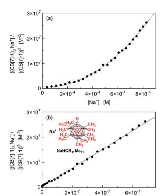
Fig. 5 (a) Plot of  $[(CB[7]\cdot 1)_3M]/[(CB[7]\cdot 1)]^3$  as a function of [M], for  $M=Na^+$  (counteranion  $CB_{11}(CH_3)_{12}^-$ ). Formation of a sodium-secured trimer should afford a linear regression, not a quadratic one. (b) Plot of  $[(CB[7]\cdot 1)_3M]/[(CB[7]\cdot 1)]^3$  as a function of [M][X], for  $M=Na^+$  and  $X=HCB_{11}(CH_3)_{11}^-$ , and linear regression.
