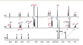
Fig. 2  $\,^{1}$ H NMR spectrum of (a) guest 1 in DMSO- $d_{6}$  (1.0 mM), (b) after addition of 1.0 equiv. CB[7], and (c) after subsequent addition of 2.3 equiv. NaCl. See Fig. 1 for hydrogen nuclei labeling. "11" and "23" exponents refer, respectively, to binary complex CB[7]·1 and to a new assembly discussed thereafter. Chemical shifts in ppm.
