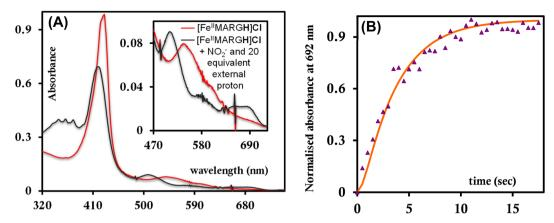
Fig. 7 (A) Absorption spectra of  $[Fe^{II}MARGH]CI$  (red) upon simultaneous addition of 5 equivalents of  $[NBu_4]NO_2$  and 20 equivalents of 2,6-xylidinium chloride (dark grey). (B) Kinetic trace followed at 692 nm regarding the formation of  $Fe^{III}$ -Cl species when nitrite and 20 equivalents of 2,6-xylidinium chloride are added to  $[Fe^{II}MARGH]CI$  simultaneously.
