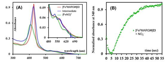
Fig. 5 (A) Intermediate absorption spectrum (blue) upon addition of [NBu<sub>4</sub>]NO<sub>2</sub> to [Fe<sup>III</sup>MARGH]Cl (red) and the corresponding final spectrum of  $\{FeNO\}^{7}$  species (green). (B) Kinetic trace followed at 540 nm for the formation of  $\{FeNO\}^{7}$  complex upon addition of 100 equivalents of  $[NBu_{4}]$ NO<sub>2</sub> to [Fe<sup>II</sup>MARGH]Cl.
