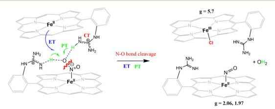
Scheme 1 A tentative description of the rate-determining ET step in the reduction of  $NO_2^-$  to  $\{FeNO\}^7$  species by  $[Fe^{II}MARGH]CI$  in the absence of external protons. The  $CI^-$  counter ion on the  $NO_2^-$  bound heme is not shown for clarity.
