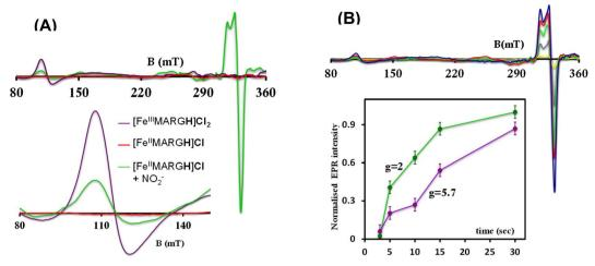
Fig. 4 (A) X-band EPR spectra of  $[Fe^{II}MARGH]Cl_2$  (violet) and  $[Fe^{II}MARGH]Cl$  (red). The green spectra correspond to the  $[FeNO]^7$  species and the ferric porphyrin generated in the reaction of [Fe<sup>II</sup>MARGH]Cl with [NBu<sub>4</sub>]NO<sub>2</sub>. (B) The corresponding spectra in different time intervals upon addition of  $[NBu_4]NO_2$  to  $[Fe^{II}MARGH]CI$  and a plot of normalized EPR intensities of the axial (violet) and rhombic (green) signals with time.
