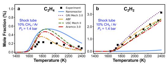
Fig. 6 Experimental and simulated (a)  $C_2H_4$  and (b)  $C_2H_2$  mole fractions. The experimental/simulation condition is 10%  $CH_4/Ar$ ,  $P_0 = 1.4$  bar, and  $t_{rec} = 2.87$  ms.
