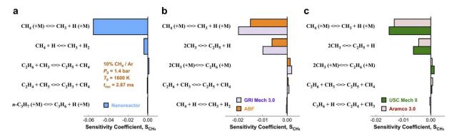
Fig. 4 Ranked sensitivity bar chart for CH<sub>4</sub> mole fraction with respect to reaction rates computed under condition 10% CH<sub>4</sub>/Ar,  $P_0 = 1.4$  bar,  $T_0 = 1600$  K, and  $t_{rec} = 2.87$  ms. Five reaction kinetic models are analyzed, including (a) the nanoreactor, (b) GRI Mech 3.0 & ABF, (c) USC Mech II & Aramco 3.0.
