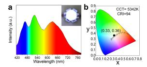
Fig. 6 (a) PL emission spectrum of a 375 nm UV-LED excited white LED device containing the as-synthesized bright and broad redemissive CsMnBr $_3$  NC embedded glasses, commercially-available blue-emissive BaMgAl $_{10}$ O $_{17}$ :Eu $^{2+}$  phosphor, and home-made greenemissive (C $_5$ H $_6$ N) $_2$ MnBr $_4$  phosphor. Inset is the lighted photograph of the WLEDs. (b) The CIE chromaticity coordinates of the white LED device shown in (a).
