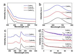
Fig. 4 (a) The UV-vis absorption spectra, (b) PL emission spectra excited at 410 nm, (c) PL excitation spectra with emission monitored at 650 nm, and (d) PL lifetime decay curves of a series of  $CsMnX_3$  (X = I, Br, CI) NC embedded glass samples.
