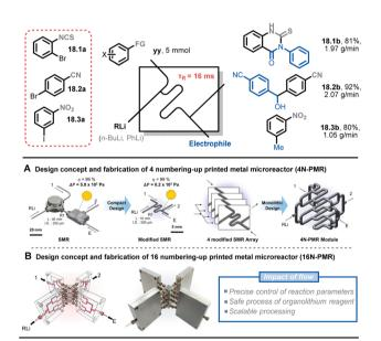
Fig. 18 Scale-up strategy for an ultrafast sub-second flash chemistry exploiting aryllithium intermediates using numbered-up 3D-printed microreactors. Reproduced from ref. 91 with the permission of American Chemical Society, copyright 2022.
