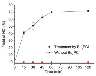
Fig. 4 Yield of HCl, determined by acid-base titration, during reaction of PVC with 0.85 eq.  $Bu_4PCl$ , 2 mol% Rh at 180 °C in butanone, with rapid dehydrochlorination during the initial 60 minutes. Error bars represent the standard deviation. Control reaction of PVC without  $Bu_4PCl$  in butanone yielded no HCl (conditions: 1 mmol PVC, 180 °C, 20 bar  $H_2$ , with 2 mol%  $H(CO)Rh(PPh_3)_3$ ).
