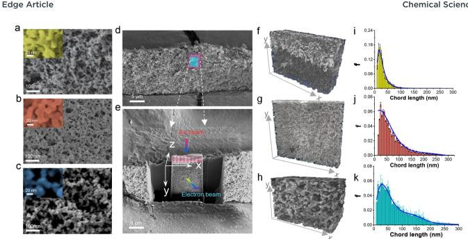
Fig. 2 Micromorphological changes during Zn precursor gel transformation to ZIF-8 and MOF-5. SEM images of the Zn precursor (a), ZIF-8 (b), and MOF-5 (c) aerogels showing highly crosslinked network structures, FIB-SEM dual beam analyses of the ZIF-8 aerogel (d and e), and the 3D reconstructed images and chord length distribution of the Zn precursor (f and i), ZIF-8 (g and j), and MOF-5 (h and k) aerogels, showing changes in their 3D micromorphology and pore interconnectivity.
