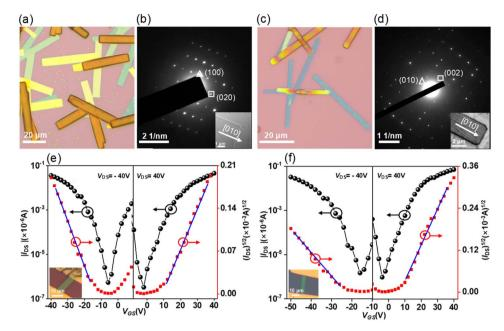
Fig. 8 Optical microscopy images of microbelts 9 (a) and  $9 \cdot C_{60}$  (c); the selected-area electron diffraction (SAED) patterns of microbelts 9 (b) and  $9 \cdot C_{60}$  (d) (inset: the TEM image of a single-crystalline microbelt); the transfer characteristics of an OFET based on microbelts 9 (W/L = 7.8/22.1) (e) and  $9 \cdot C_{60}$  (W/L = 4.8/23.3) (f).
