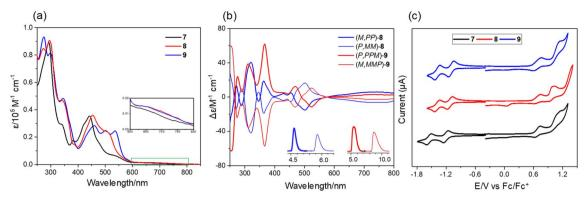
Fig. 5 (a) UV-vis absorption of 7–9 in chloroform ( $\sim$ 10<sup>-5</sup> M); (b) CD spectra of the enantiomers of 8 and 9 in chloroform. (inset: resolution of the enantiomers of 8 and 9 by chiral analytical HPLC.); (c) cyclic voltammograms of 7–9 in nitrogen-purged dichloromethane with tetrabutylammonium hexafluorophosphate (TBAPF<sub>6</sub>, 0.1 M) as the supporting electrolyte and a scan rate of 100 mV s<sup>-1</sup>.
