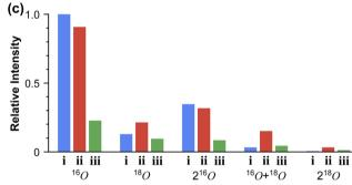
Fig. 8 Measurement using the oxygen isotope. (a) Mass spectra obtained under oxidized conditions for 5 µM L-phosphatidylcholine (PC 18:1/18:1) in 500 mM HCl prepared using normal water (i) and water-<sup>18</sup>O (ii & iii). The operating gases are air (i & ii) and high-purity nitrogen (iii). Asterisk denotes the peak without oxidation. (b) Enlarged view of (a) (i) and (a) (ii). (c) Intensity comparison for different oxidation species.
