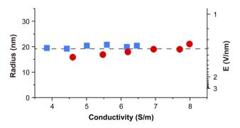
Fig. 4 Threshold electric field. Radius and the electric field of the initial droplet at the threshold for the detection of oxidized species. The sample is cytochrome c (25  $\mu$ M) in different buffer solutions of various electrical conductivities. Blue square: ammonium acetate. Red circle: ammonium formate. The average threshold radius and electric field are  $\sim$ 19.2 nm and 1.3 V nm $^{-1}$ .
