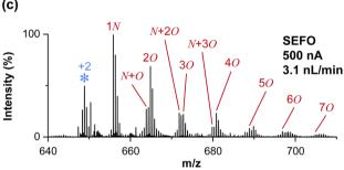
Fig. 7 Oxidation by ozone. (a) Oxidation of 10  $\mu$ M melittin in 100 mM ammonium formate using ozone produced from the DBD source. (b) Oxidation of 20 µM angiotensin I in 50 mM HCl using ozone. (c) Strong electric field-induced oxidation of angiotensin I in 500 mM HCl. Asterisk denotes the unoxidized peak.
