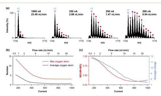
Fig. 2 Cytochrome c in 1 M ammonium formate. (a) Mass spectra of cytochrome c (25  $\mu$ M) in 1 M ammonium formate aqueous solution acquired at different spray currents. The red solid circle denotes the oxidized peak. Asterisk denotes the unoxidized peak. (b) Maximum (red) and the average (solid) number of oxygen atoms *versus* spray current. (c) Ratio of total oxidized ion species to the total ion signal (red) and the average charge state (blue) *versus* spray current.
