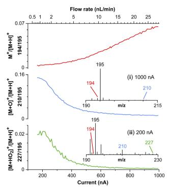
Fig. 5 Detection of caffeine molecular ion. Detection of caffeine (25  $\mu$ M) in 200 mM HCl under different spray currents. Red: Intensity ratio of  $M^{+}/[M + H]^{+}$ . Blue:  $[M + O]^{+}/[M + H]^{+}$ . Green:  $[M + HO_{2}]^{+}/[M + H]^{+}$ . Mass spectra in the inset are taken at 1000 and 200 nA.
