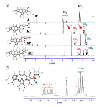
Fig. 3 Comparison of the <sup>1</sup>H NMR spectra of (a) secoHPHAC 2 (in CDCl<sub>3</sub>) and homoHPHAC  $3c^+-3e^+$  (in acetone- $d_6$ ), and (b) an enlarged view of the spectrum of 3e+.
