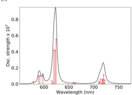
Fig. 3 Computational analysis of 5-PP-InsP<sub>5</sub> binding to [Eu.3]<sup>+</sup>: (a) DFT optimised geometry of the bidentate binding mode and (b) *ab initio* luminescence spectrum from  $^5D_0$  showing the individual microstates of the  $^7F$  term as red crosses on lines proportional to their oscillator strength.
