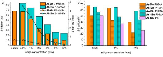
Fig. 4 (a) Z-Fractions upon excitation with 660 nm light and thermal Z half-lives of Al-Me and Al-tBu, and (b) Z-fractions of Ar-Me, As-Me, Ar-tBu and As-tBu at different dye loadings in PHMA and Ar-tBu in PS.
