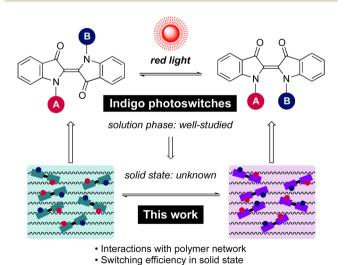
**Scheme 1** E-Z isomerisation of indigo photoswitches and the focus of this work.
