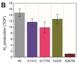
Fig. 4 (A)  $H_2$  oxidation activity (s<sup>-1</sup>) for the TmHydS variants measured at 70 °C in 200 mM phosphate buffer pH 8 under a 100%  $H_2$  atmosphere following 1 mM benzyl viologen reduction using UV-vis absorbance at 600 nm. (B)  $H_2$  production activity (s<sup>-1</sup>) measured at 70 °C with gas chromatography after 10 min of incubation with 100 mM sodium dithionite and 10 mM methyl viologen.
