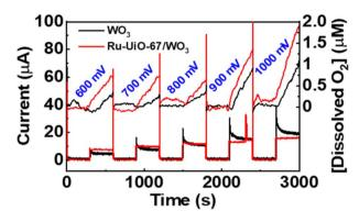
Fig. 8 Current increase (bottom) and  $O_2$  production (top) for  $WO_3$  and Ru-UiO-67/ $WO_3$  at different applied potentials. At each potential, the photoelectrode was held in the dark for 5 minutes before illumination for 5 minutes.
