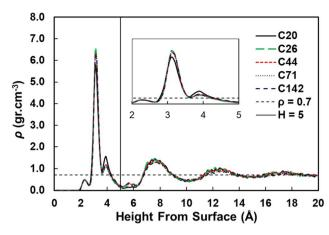
Fig. 2 Density distributions as a function of the distance from the Pt(111) surface for pure PE surrogates. The inset shows the zoom in region from 2 to 5 Å from the surface.
