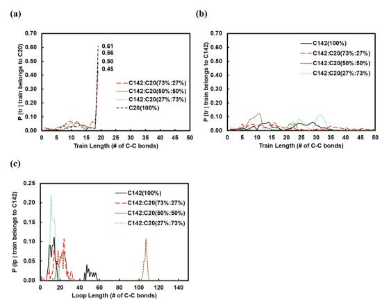
Fig. 6 Conditional probability of the length of the trains in (a)  $C_{20}$  chains and (b)  $C_{142}$  chains. (c) Conditional probability of the length of the loops in  $C_{142}$  for  $C_{142}$ :  $C_{20}$  mixtures of varying concentrations over Pt(111) at 473 K. Adsorbed  $C_{20}$  chains do not form loops.
