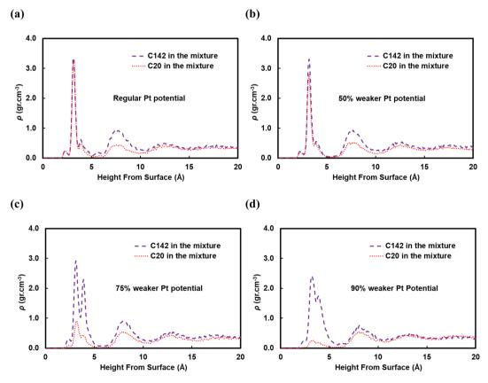
Fig. 9 Density profiles of a binary mixture of  $C_{20}$  and  $C_{142}$  with 50 wt%  $C_{20}$  for a (a) regular, (b) 50% weaker, (c) 75% weaker, and (d) 90% weaker Pt potential showing long chain segregations by decreasing the Pt potential strength.
