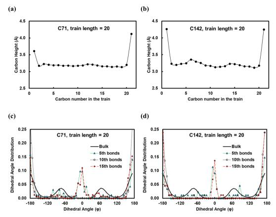
Fig. 5 (a) and (b) Average distance of carbons in a train length of 20 from the Pt(111) surface for the  $C_{71}$  and  $C_{142}$  melts, respectively. (c) and (d) Distribution of the torsion angle about the 5th, 10th and 15th bonds of the train for the  $C_{71}$  and  $C_{142}$  melts, respectively.
