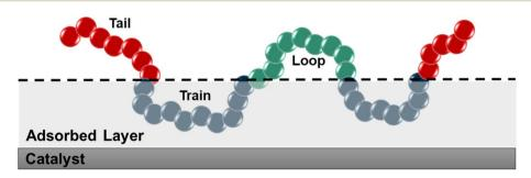
Fig. 1 Schematic representation of trains (blue), tails (red), and loops (green). The thickness of the adsorbed layer was set to 5 Å, which was defined using the density distribution in Fig. 2.
