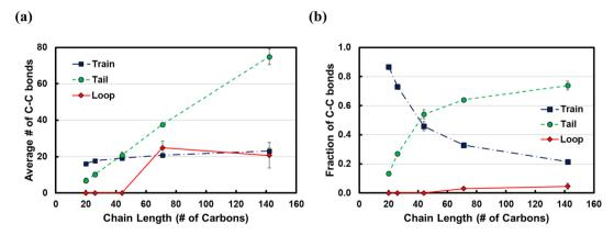
Fig. 4 (a) Average length of trains, tails and loops in number of carbons and (b) fraction of C-C bonds of adsorbed chains belonging to trains, tails, or loops as a function of the chain length at 473 K. Error bars represent one standard deviation.
