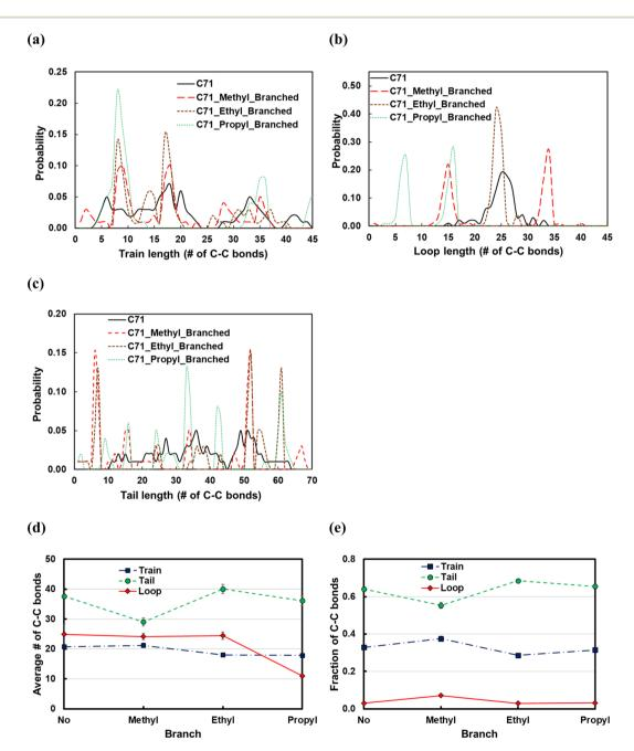
Fig. 11 Dependence of (a) train size distributions, (b) loop size distributions, (c) tail size distributions, (d) average length of trains, tails, and loops, and (e) fraction of C-C bonds in trains, tails, or loops on the length of side chains in the  $C_{71}$  backbone. Error bars represent one standard deviation.
