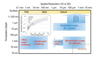
Fig. 1 Typical penetration depth and spatial resolution (1D and 2D measurements) for selected analytical techniques. The inset depicts 1/e penetration depths for various battery relevant materials as a function of energy (E), where e is Euler's number. TEM and SEM stand for Transmission Electron Microscope and Scanning Electron Microscope, respectively. Reproduced from ref. 6 with permission, © Materials Research Society.
