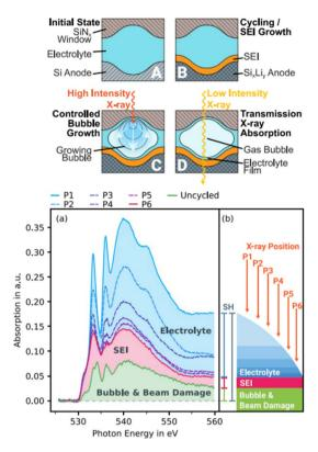
Fig. 5 (a) Illustration of a novel approach to investigate the SEI on silicon thin-film electrodes in situ through transmission sXAS and (b) extraction of the SEI spectrum from the overshadowing electrolyte spectrum and subtraction of the bubble and beam damage.82
