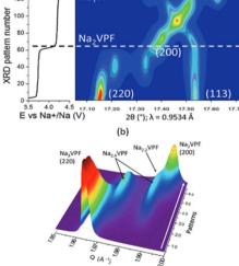
Fig. 2 Image of a thermalized cell<sup>21</sup> designed taking the one reported in ref. 22 as the basis, modified to enable fluid circulation through the main cell body (top). Diffraction patterns achieved using a similar setup for Na $_3$ V $_2$ (PO $_4$ ) $_2$ F $_3$  in sodium cells at C/10 and 0 °C, which enabled the phase diagram to be followed upon Na $^+$  deintercalation in 2D (a) and 3D (b) plots. Reproduced from ref. 23 with permission, © WILEY-VCH Verlag GmbH & Co.
