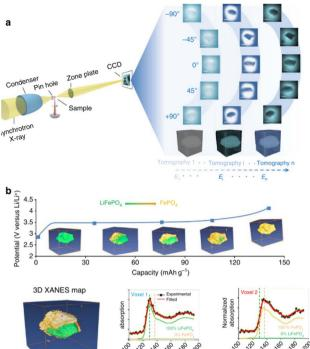
Fig. 11 Illustration of a 5D Fe K-edge XANES tomography. (a) Schematic of the experimental setup. A tomography data set is collected at different energies across the near Fe K-edge absorption to access chemical information for each voxel. By fitting the resulting spectra as a linear combination of spectra of end-phases, phase composition can be assigned to each voxel (right side). (b) Chemical phase distribution as a function of capacity (proportional to time). Reproduced from ref. 154
