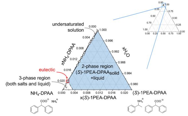
Fig. 6 Ternary phase diagram of the ammonium/(S)-1PEA-DPAA salt pair in 10 mM phosphate buffer, pH 7.5.
