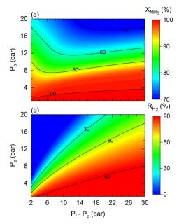
Fig. 11 Contour plots of membrane reactor performance using Co- $Ba/CeO_2$  as a function of permeate  $(P_p)$  and transmembrane differential pressure  $(P_f - P_p)$  in terms of (a) NH<sub>3</sub> conversion and (b) H<sub>2</sub> recovery. Simulation conditions: estimated kinetic, membrane, and heat transfer parameters (Table 4) and  $T_{\text{wSP}}$  = 450 °C; W = 20  $g_{\text{cat}}$ ;  $W/F_0 = 22 g_{cat} h mol^{-1}$ .
