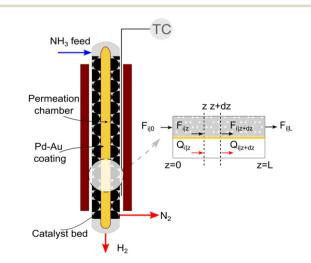
Fig. 1 Schematic and sectional view of the catalytic packed bed membrane reactor used for ammonia decomposition.
