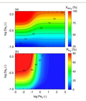
Fig. 2 Effect of Damköhler (Da) and Peclet (Pe) numbers on (a) NH<sub>3</sub> conversion and (b) H<sub>2</sub> recovery. Simulation conditions: St =  $\infty$ ;  $P_r$  = 4;  $P_p$  = 1 bar;  $T_w$  = 400 °C;  $T_0/T_w$  = 1;  $\alpha_{\text{H}_2/\text{NH}_3}$  = 10<sup>5</sup>;  $\alpha_{\text{H}_2/\text{N}_2}$  = 10<sup>5</sup>; a = 0.5; b = -0.75; n = 0.5.  $X_{\text{eq@400°C}}$  = 99.8%.
