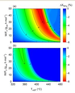
Fig. 10 Contour plots of NH<sub>3</sub> conversion loss using Co-Ba/CeO<sub>2</sub> with variable wall temperature compared to constant wall temperature  $(T_0)$  $T_{\rm w}$  = 1) in terms of wall temperature setpoint and space-time for (a) non-membrane reactor and (b) membrane reactor. Simulation conditions: estimated kinetics, membrane reactor, heat transfer parameters (Table 4), and  $F_{NH_{z},0} = 1 \text{ N mL min}^{-1}$ ;  $P_r = 10$ ;  $P_p = 1 \text{ bar.}$
