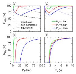
Fig. 4 Permeate pressure effect on NH<sub>3</sub> conversion for different (a) feed pressures  $(P_f)$  and (b) pressure ratios  $(P_r)$ ;  $H_2$  recovery for different (c) feed pressures  $(P_f)$  and (d) pressure ratios  $(P_r)$ . Simulation conditions: Da/ $P_f^{(a+b)} = 1$ ; Pe ×  $P_f^n = 0.05$ ; St =  $\infty$ ;  $T_w = 400$  °C;  $T_0/T_w$ = 1;  $\alpha_{\text{H}_2/\text{NH}_3}$  = 10<sup>5</sup>;  $\alpha_{\text{H}_2/\text{N}_2}$  = 10<sup>5</sup>; a = 0.5; b = -0.75.
