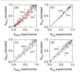
Fig. 5 Comparison of experimental values and simulation predictions after parameter estimation of (a) set (i) (Ru–K/CaO, black squares: Co–Ba/CeO<sub>2</sub>, red circles); (b) set (ii); and (c) and (d) set (iii) in terms of NH $_3$  conversion and H $_2$  recovery, respectively.
