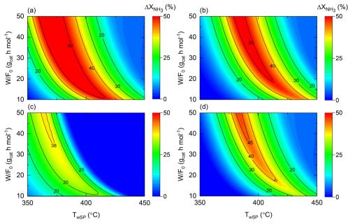
Fig. 9 Contour plots comparing NH<sub>3</sub> conversion enhancement as a function of space-time  $(W/F_0)$  and wall setpoint temperature  $(T_{WSP})$  for cases (a) 3 vs. 1; (b) 4 vs. 2; (c) 3 vs. 4; and (d) 4 vs. 1. Simulation conditions: estimated kinetic, membrane, and heat transfer parameters (Table 4) and W  $= 20 g_{cat}$ ;  $P_r = 10$ ;  $P_p = 1 bar$
