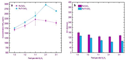
Fig. 7 Effect of different feed gas ratios on (a) NH<sub>3</sub> concentrations and (b) ECs. Reproduced from ref. 70 with permission from Elsevier B.V., copyright 2023.
