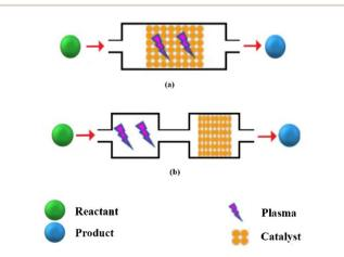
**Fig. 4** Two types of plasma-catalysis reactors (a) single-stage system (b) two-stage system.
