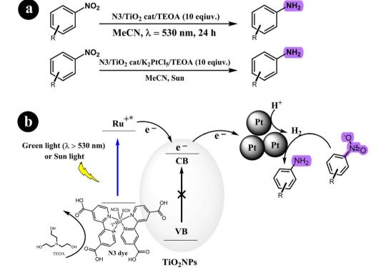
Scheme 14 (a) Reaction condition for the conversion of nitroarenes to anilines and (b) the proposed mechanism involving the reduction of nitroarenes using a green-light/sun light mediated process facilitated by dye-sensitized TiO2 and transition metal clusters. TEOA (triethanolamine) is also involved in the reaction. Reproduced from ref. 55 with permission, copyright 2010, Royal Society of Chemistry.
