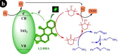
Scheme 26 (a) 1,2-DHA- $TiO_2$ /TEMPO co-catalyst for the green light-induced photocatalytic selective oxidation of primary and secondary amines into imines using aerobic  $O_2$  as the oxidizing agent, and (b) the proposed mechanism for the reactions. Reproduced with permission from ref. 76, copyright 2021, Elsevier.
