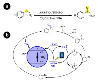
Scheme 6 (a) Reaction conditions and (b) possible mechanism for the oxidation of sulfides to sulfoxides by ARS-TiO2 under blue LED irradiation. Reproduced with permission from ref. 41. Copyright 2018, John Wiley and Sons.
