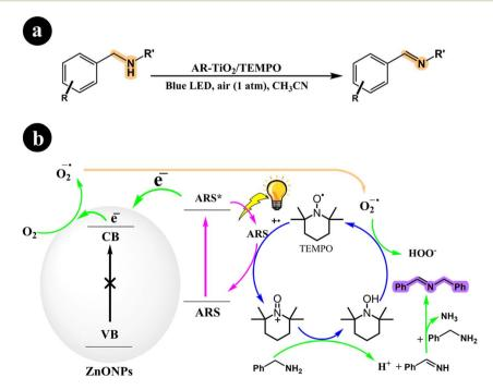
Scheme 9 (a) Reaction conditions for the aerobic oxidation of amines to imines by ARS- $TiO_2$  using  $O_2$  with TEMPO under blue light irradiation and (b) mechanistic pathway. Reproduced with permission from ref. 47, copyright 2018, Elsevier.
