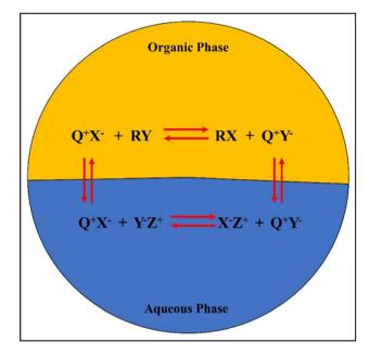
Fig. 8 Mechanism of PTC in a biphasic mixture.
