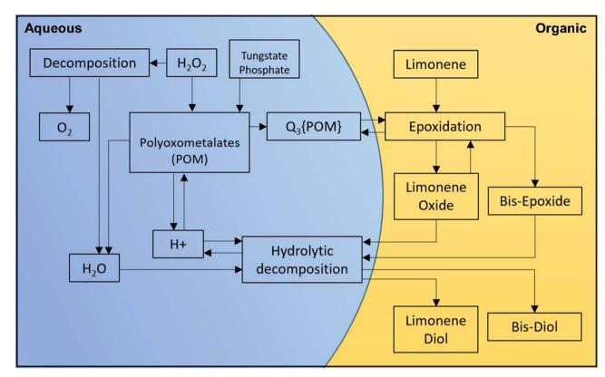
Fig. 5 Overall reaction scheme for the epoxidation of (R)-(+)-limonene, the formation of oxidative species, the decomposition of  $H_2O_2$  and the hydrolytic decomposition of the epoxides. Each reaction is visualized in the schematic diagram (an aqueous phase is shown in blue, while an organic phase is shown in gold).
