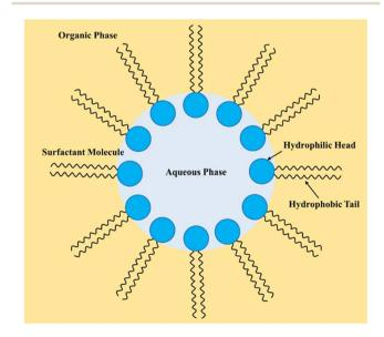
Fig. 7 Schematic of a 'water-in-oil' emulsion where the hydrophobic tail of the surfactant stretches towards the organic phase (gold background). In the meantime, the hydrophilic head remains in the aqueous phase (blue background).
