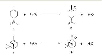
Scheme 2 Epoxidation of terpenes with  $H_2O_2$ . (1) (R)-(+)-limonene, (2) trans-limonene-1,2-epoxide, (3)  $\alpha$ -pinene and (4) trans- $\alpha$ -pinene oxide.
