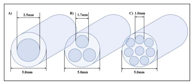
Fig. 11 Orifice meso-OBR design schematics and configurations for 3D printing, (A) single orifice (B) tri-orifice (C) Multi-orifice.<sup>5</sup>
