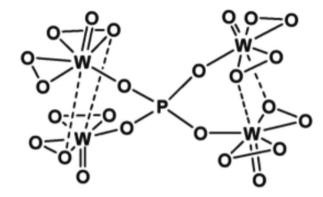
Fig. 4 The visualisation of the structure of Venturello anion (PW<sub>4</sub>).<sup>116</sup>
