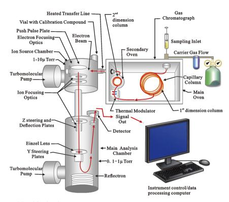
Fig. 8 Schematic diagram of GC  $\times$  GC-TOFMS-instrument.
