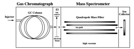
Fig. 7 Schematic diagram of GC-MS.
