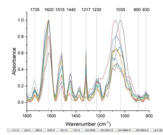
Fig. 3 FTIR spectra of all 11 samples are displayed for the fingerprint region of  $800-1800 \text{ cm}^{-1}$ . All spectra were baseline corrected and normalized between [0,1]. Specific wavenumbers of interest are indicated on the x-axis, such as 830 cm<sup>-1</sup> for syringyl units (827–833 cm<sup>-1</sup>) and 910 cm<sup>-1</sup> for quaiacyl units (908–913 cm<sup>-1</sup>).
