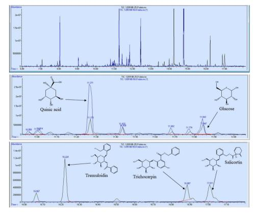
Fig. 5 GC/MS chromatogram of two selected samples: LILC-26-4-S (black) and 1031-N (blue). The retention time periods of approximately 11–12 minutes and 16–17 minutes have been enlarged to detail differences in metabolites such as quinic acid, glucose, tremuloidin, trichocarpin, and salicortin.
