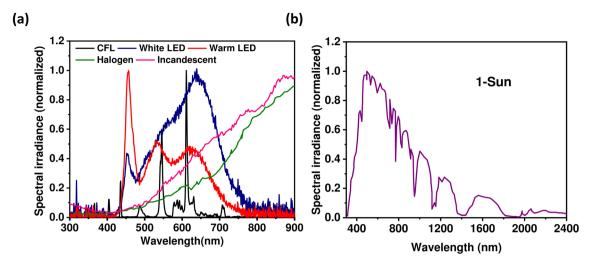
Fig. 1 (a) Irradiance spectra of different indoor light sources;<sup>16</sup> (b) solar spectra (AM1.5G).<sup>16</sup>
